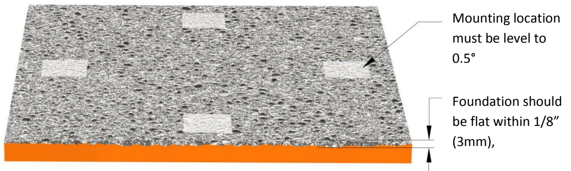
Figure 06 : Foundation for weighing module installation.
