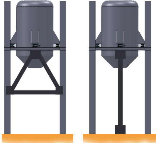
Figure 13 : Typical reinforcement methods for support beams
