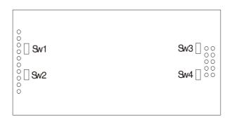
Sw1 & Sw2 : Close for 4-wire loadcell Sw3 : Close to enter configuration mode Sw4 : Do NOTclose - used for program download
