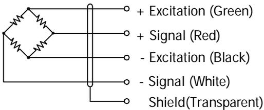
Cable : 22AWG, 4-conductor AL foil shielded cable with drain.
