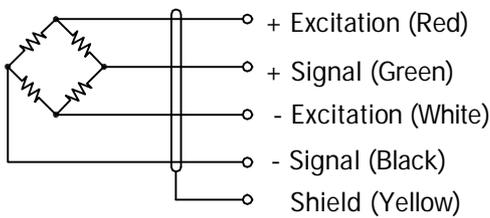
Cable : 28 AWG, 4 Conductor braided shield cable .
