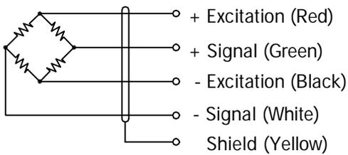
Cable : 24 AWG. 4-Conductor PU gray cable.
