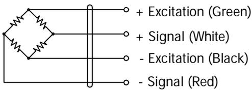
Cable : 28 AWG, 4 Conductor cable with shield.
