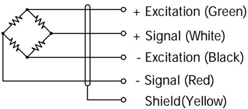
Cable : 24AWG, 4 Conductor cable with shield.
