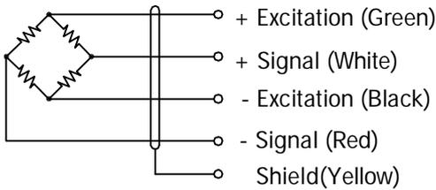
Cable : 24AWG, Foil shielded, 4 Conductor cable.
