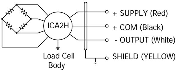
Cable : 24 AWG, 4 conductor cable with shield
