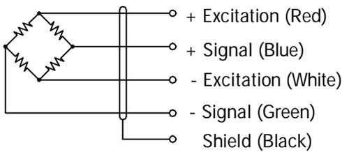
Cable : 24 AWG, 4 Conductor shielded cable.
