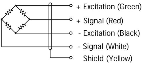
Cable : 24 AWG, 4-Conductor AL foil shielded black cable.
