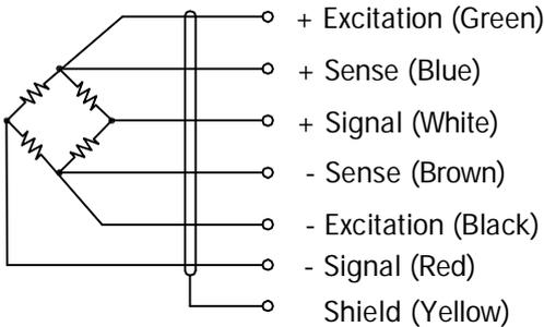
Cable : 24 AWG, 6 Conductor cable with shield.
