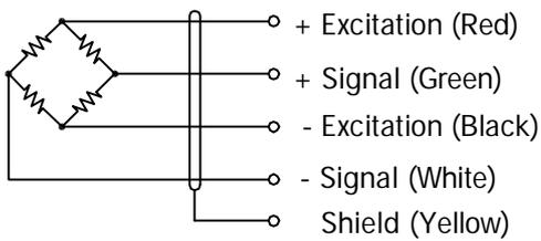
Cable : 28 AWG, 4 Conductor cable with shield.
