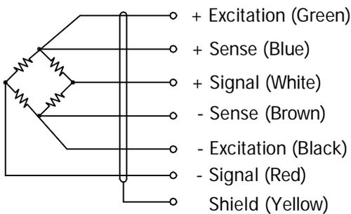
Cable : 26 AWG, 6 Conductor with Shield.
