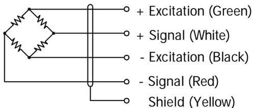
Cable : 24 AWG, 4-Conductor shielded cable with polyurethane jacket.
