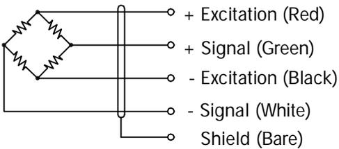
Cable : Ø5.1mm, 4 Conductor cable (Capacity ≤20Klb).
