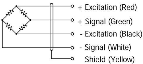
Cable : 28AWG, 4 conductor gray cable with shield.
