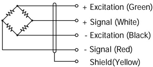
Cable : 20AWG, 4 Conductor cable with shield.
