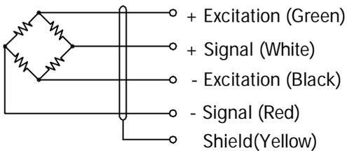
Cable: 20 AWG, 4-conductor with shield
