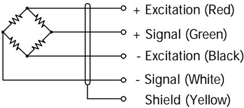
Cable : 20 AWG, 4 Conductor black cable with shield.
