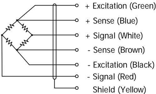
Cable : 24 AWG, 6 Conductor with shield.
