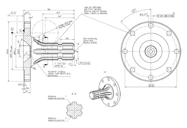
PTO shaft 6 teeth (1 3/8"), ≤ 2.500 Nm maximum dynamic constant load
