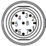
M8, A CODING 8PIN MALE CONNECTOR PIN CONFIGURATION
