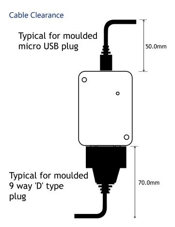
These are typical clearances but smaller mouldings or using a tighter cable radius can reduce this.
