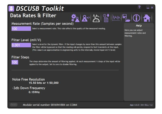
This page allows you to select the measurement rate and filtering characteristics.
