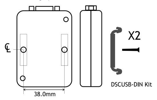
A DIN rail mounting kit is available for top hat DIN rail EN 50022. Optional part DSCUSB-DIN consists of a pair of screws and two DIN rail clips.
