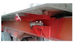
On-board vehicle weighing, on-board weighing on vehicles and agricultural machinery
