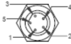
M8, 5 PIN FEMALE CONNECTOR
